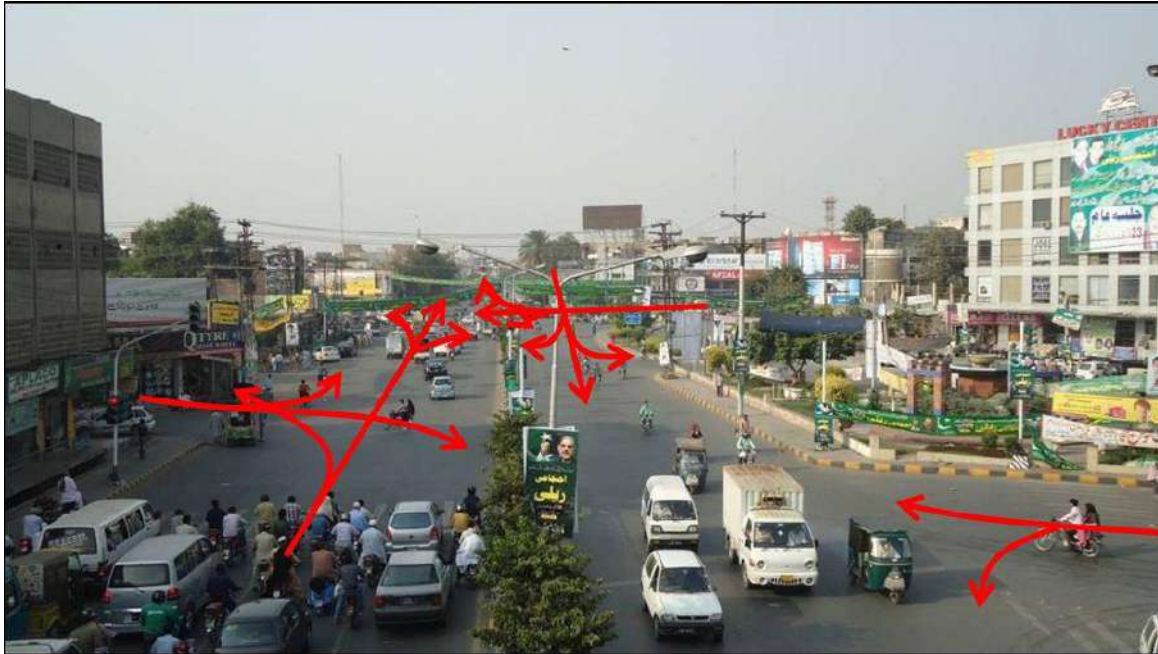
Figure 8.5.1 Poor Traffic Circulation at Qurtaba Chowk – Note Conflicting Movements
